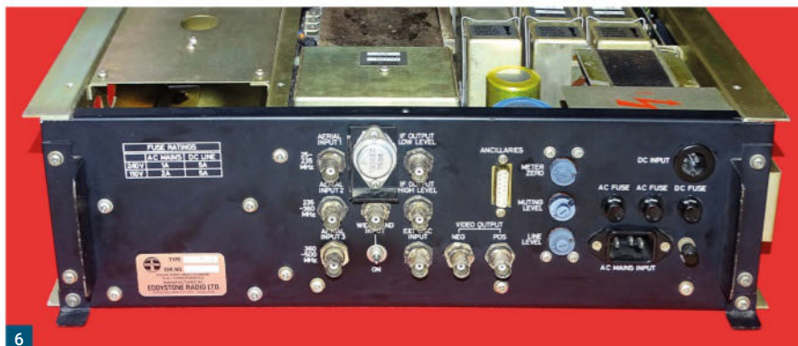
Fig. 6: The rear panel carries three antenna inputs as well as outputs for several ancillaries. Fig. 7: The VHF tuner incorporates a dual-gate MOSFET RF amplifier and a diode quad balanced mixer. Fig. 8: The tuning gearbox drives a 10-turn potentiometer as well as the 4-gang variable capacitor in the VHF tuner.
